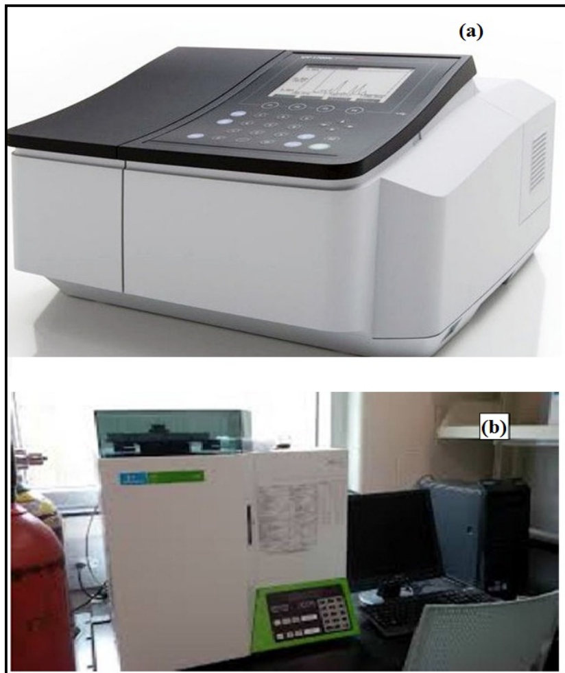
Figure 6: Photographic images of (a) Shimadzu spectrophotometer model UV-1200; (b) Thermo Finnigan Elemental Analyzer
